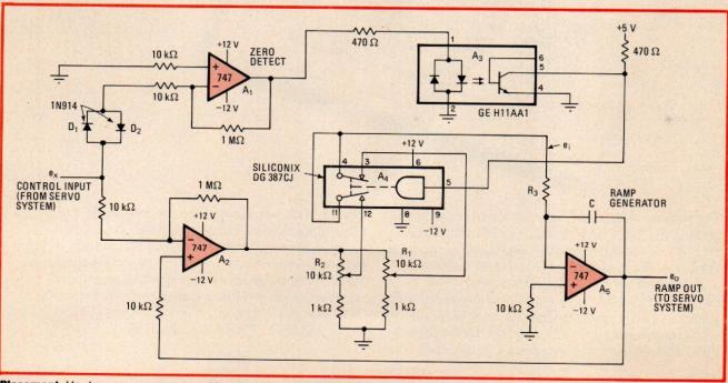
Placement. Up-down ramp generator with selectable-slope capability can efficiently position heavy servo-system loads. Key to operation is solid-state relay A<sub>4</sub>, which switches from up ramp to down ramp to decelerate load when it zeros in on terminating position.
